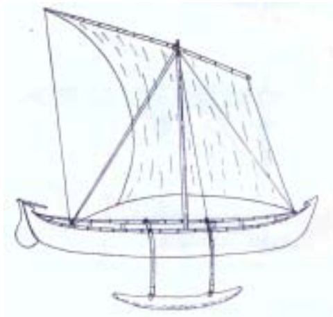
Fig 6- A Kilakarai outrigger fishing-boat, with two booms
