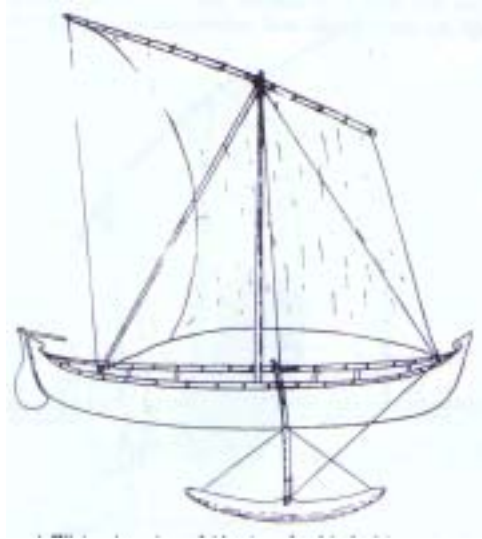
Fig 7- A Kilakarai outrigger fishing-boat furnished with one boom only
