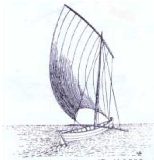
Fig 8 - A balance-board fishing canoe of Tirupalakudi, Palk Bay
